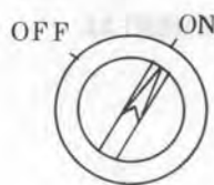
REFERENCE POINT RETURN Switch
